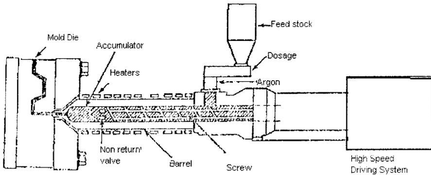
*Figure 1. Semi-solid injection molding machine.*
